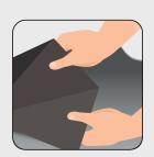
7. A self-adhesive, reinforcement kit is provided. Cut reinforcement patch to size desired, reel backing from patch material (see photo) and place it onto the underside of the cover. Reinforcement the material should be placed in areas where sharp edges could possibly cut or wear a cover, such as the corners of T-Top, windshields, trolling motors, etc.
