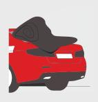
**2** Carefully remove your SealSkin Cover from the carrying case on the top of your vehicle with the front of the cover facing the front of your vehicle, being careful it does not touch the ground. We suggest beginning towards the rear of your vehicle.
