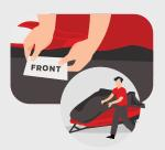
2 Find the label with arrows sewn into the hem of the cover-this is the front of your cover. Now stretch the cover down over your jet ski, ensuring the front struts are covered. Straps and buckles secure the cover's front corners to the sled's mounts. Find these straps and buckles, run the male pin around each strut, and clip it to the corresponding female buckle. Pull the strap tight to secure it.
